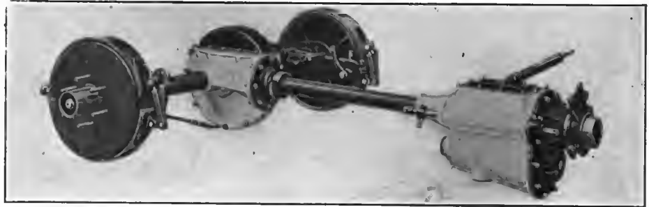
Transmission and rear axle construction showing new style brakes
